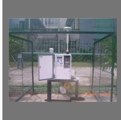
Ambient Air Quality Monitoring System
