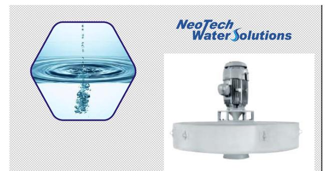
The NeoMax Hx aerator is a high speed floating mechanical aerator for wastewater treatment. Powerful pumping action transfers oxygen by breaking up the wastewater into a spray of particles, creating more surface area for atmospheric pressure to drive oxygen into the wastewater. At the same time, the oxygen enriched water is dispersed and mixed.
