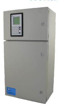
MICROMAC TOC analyzer has been designed for the automatic measurement of total organic carbon in water, on different types of matrix, using the EPA approved method based on UV persulfate oxidation and detection of generated carbon dioxide using a Non Dispersive Infrared Analyzer. This method also meets requirements of European ISO/CEN guidelines; the analyzer is conformed to EPA, DIN, CE, ASTM, NAMUR regulations.
