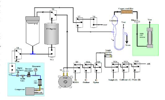
Halogen filter is used to prevent corrosion and condensation inside the stainless steel NDIR flow cell. Compressed air is scubbered in a soda lime filter, to have a free carbon dioxide gas carrier available. Carrier flow is controlled by a pressure regulator; the flow regulator and the flow rate is measured and displayed by a digital flowmeter.
